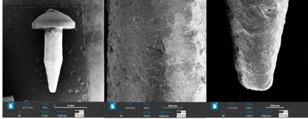
Figure 1 - General view, surface finish and detail of nail tip
